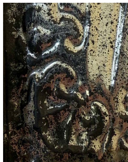
Il. 2. A fragment of a visual analysis of the product, revealing signs of galvanic coating of the tombak base, the former being distinguished by a characteristic shine, and the latter by traces of corrosion
